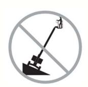
Do not use the tilt alarm as a level indicator. The tilt alarm sounds in the platform only when the machine is on a severe slope.
