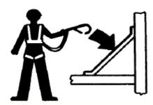
a) Occupants must wear a safety belt or harness in accordance with governmental regulations. Attach the lanyard to the anchor provided in the platform.
