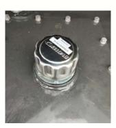
Figure 5-5 Hydraulic Tank Breather
