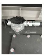
Figure 5-4 Hydraulic return filter
