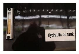
Figure 5-2 Hydraulic oil tank scale
