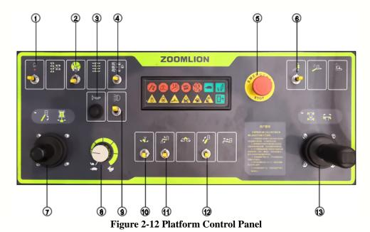
$(The \ switch \ number \ corresponding \ to \ the \ existing \ function \ has \ been \ identified.)$
