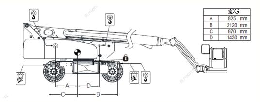
**Figure 4-1 Lifting and Securing Instructions**
