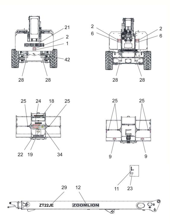
Figure 3-1 Decal Position (continuous)
