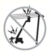
Do not operate the machine during lightning or storms.
