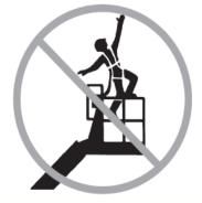
b) Do not sit, stand or climb on the platform guard rails. Maintain a firm footing on the platform floor at all times.
